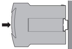
Fig.2 Mounting onto top-hat rail 35 x 15 or 35 x 7.5 mm.
