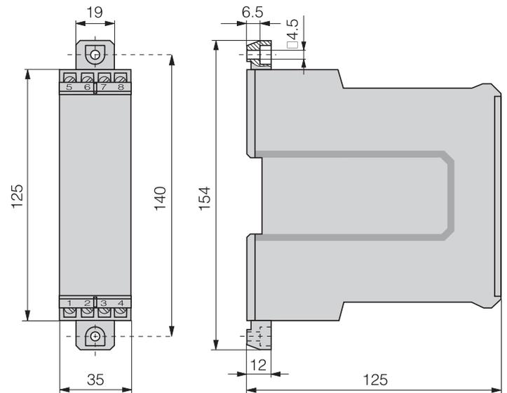
Fig.7 Transducer with the screw hole brackets pulled out for wall mounting
