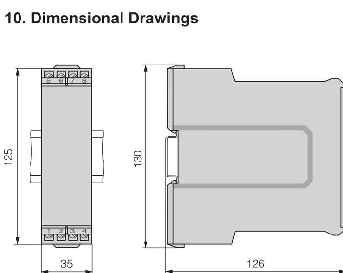
Fig.6 Transducer clipped onto a top-hat rail (35 x 15 mm or 35 x 7.5 mm) acc. to EN 50022
